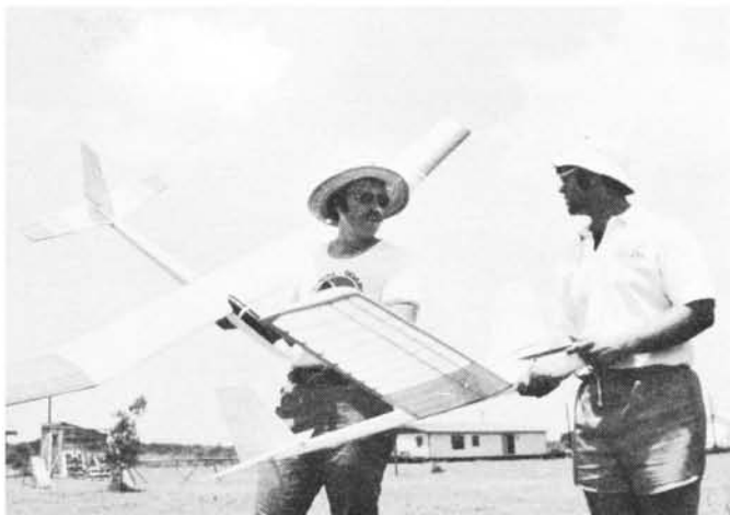
Bill Mueller, of Hi-Flight winch fame, with Scott Simmons and their Mirages. The Blaine Rawdon design is a real lightweight. Having rudder and elevator, and a 114-in. wing with 923 squares, it weighs 35 oz.
